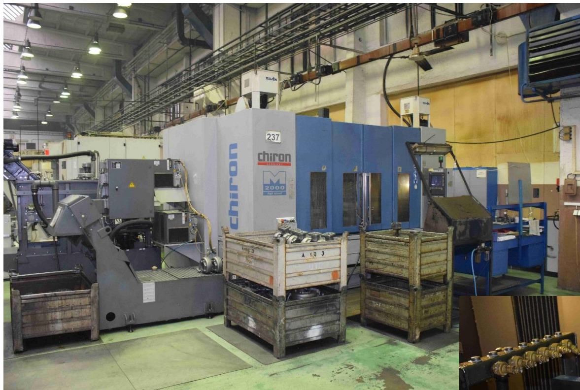
Chiron Mill 2000 – machining of turbine housing
