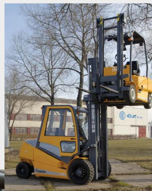
The outfit of the D (G) 40 - 50 series trucks with double tyres on the front axle, together with an optional differential lock, enable their use on soft surfaces, material handling on building sites and in other demanding conditions.
